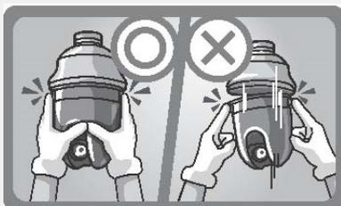
2. To protect the glass dome from getting dirty and scraped up, please put on the supplied gloves before installing.
