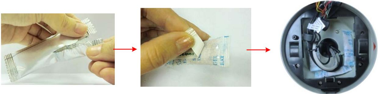
**Note:** Ensure **Not** to place the desiccant bags under the position of the fan.
